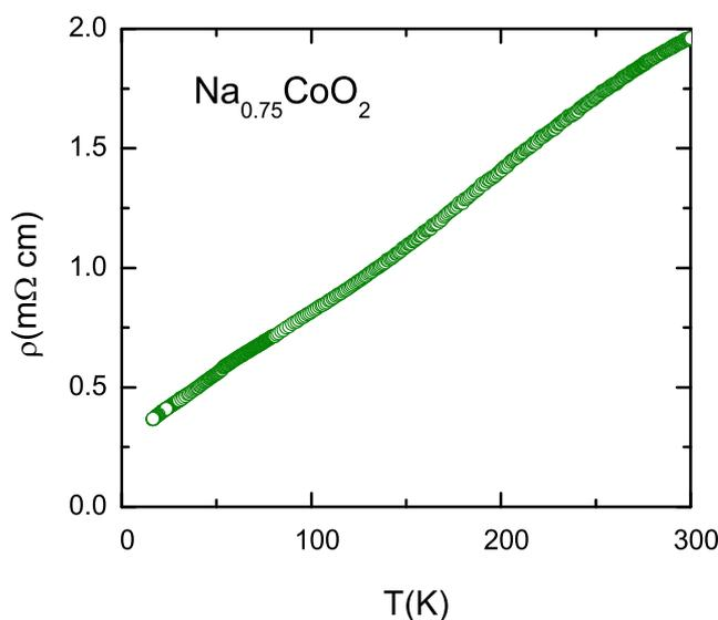
Figure 2: Temperature dependence of resistivity of  $\text{Na}_{0.75}\text{CoO}_2$ .
