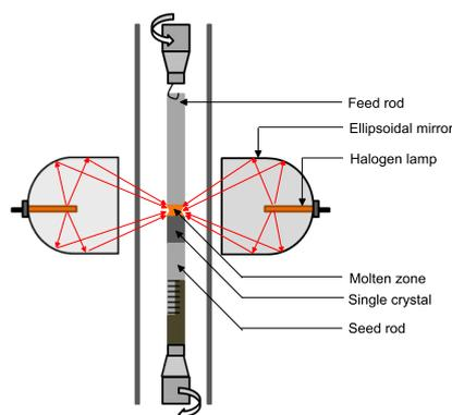
Figure 1: Schematic diagram of the floating zone technique.
