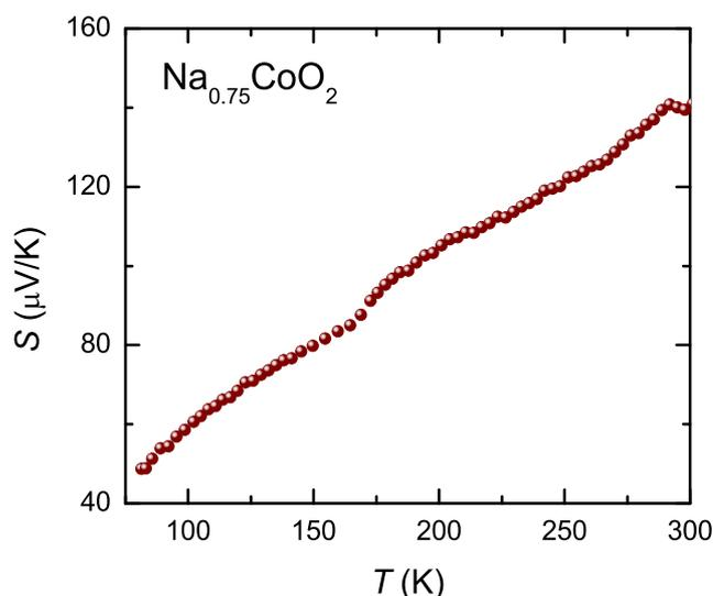
Figure 3: Thermoelectric power ( $S$ ) vs. temperature ( $T$ ) for  $\text{Na}_{0.75}\text{CoO}_2$ .
